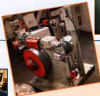
3116" HARTFORD 3-350, 2" c/o, 1-1/4" under head, PKO, 350 ppm, 1 plane straightener, ref # 22039
